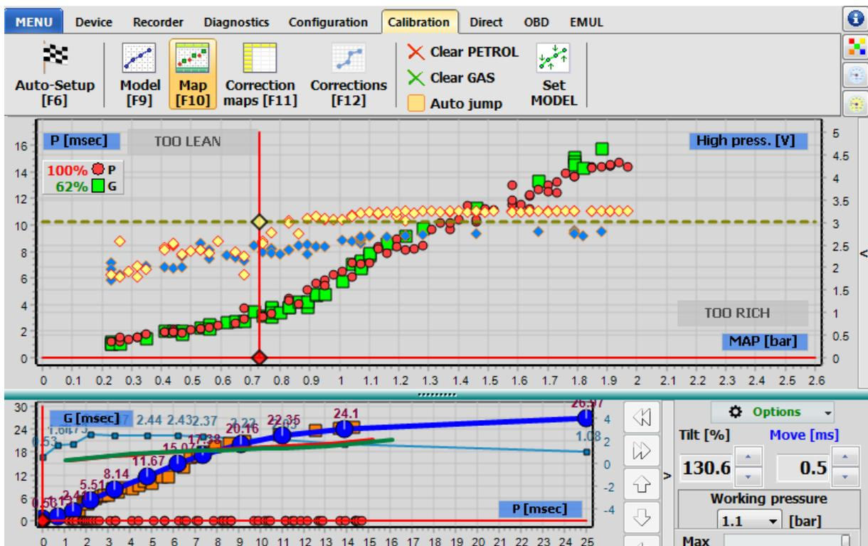
Fig. 2.78 Map window in the Calibration tab
