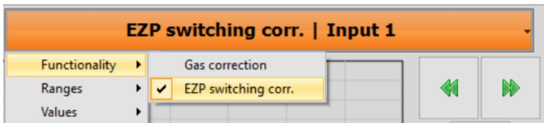
Fig. 2.90 turning on EZP correction
